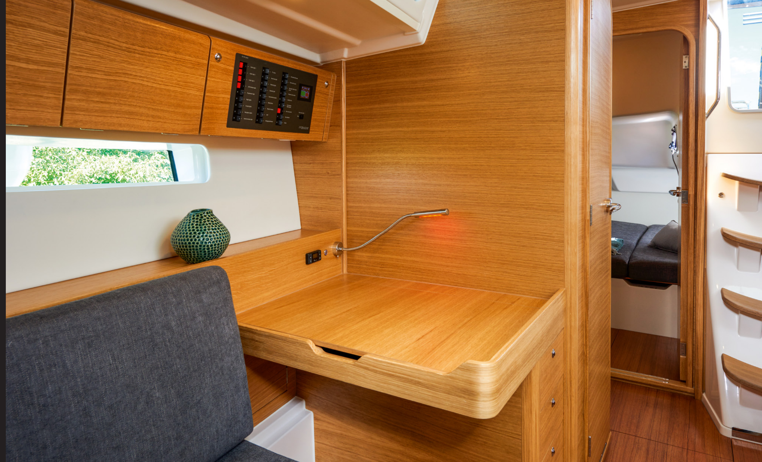
Left and top right: The Xp 44 features a sliding navigation station as standard, shown here in forward position
