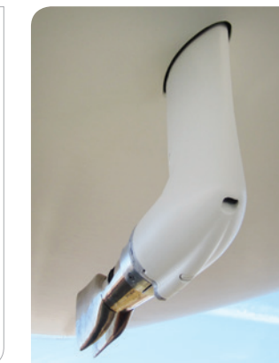
X-Yachts engine struts are faired into the hull for reduced drag and improved reliability
